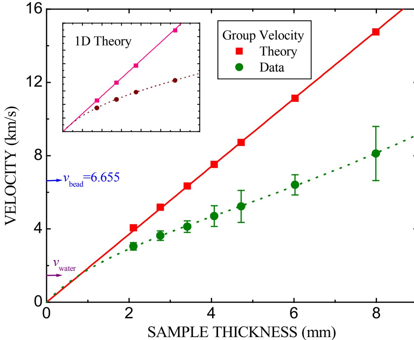
Add: the phase velocity in the middle of the gap for the same sample thicknesses.
