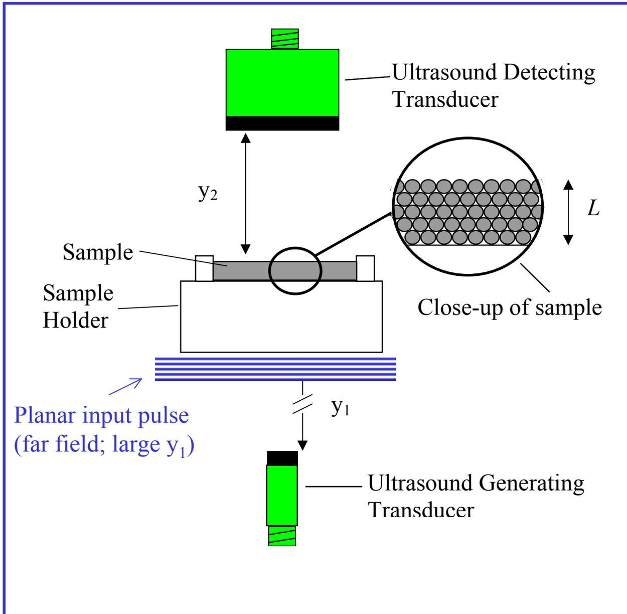
Compare transmitted pulses with reference pulses to measure:
