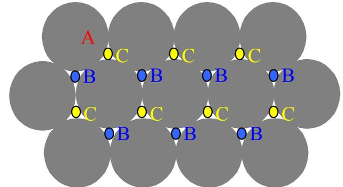
Schematic graph shows how the beads are packed in a FCC crystal along the  $[111]$  direction. Beads **A** are on the bottom layer, **B** the second and **C** the third. The sequence is **ABCABC...**
