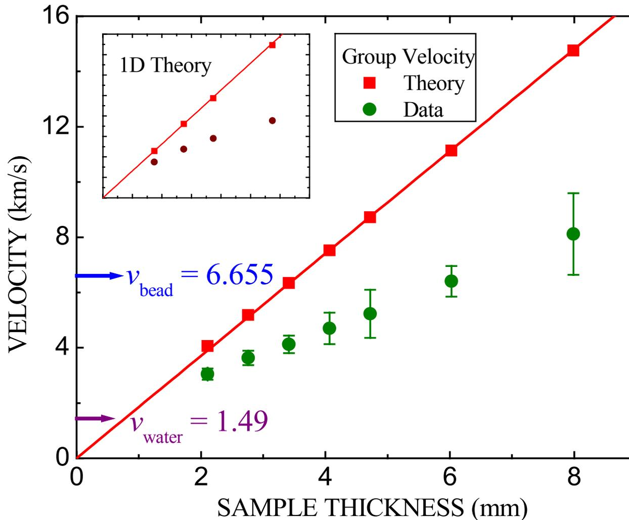
The group velocity increases linearly with thickness!  $\Rightarrow$  tunneling.
